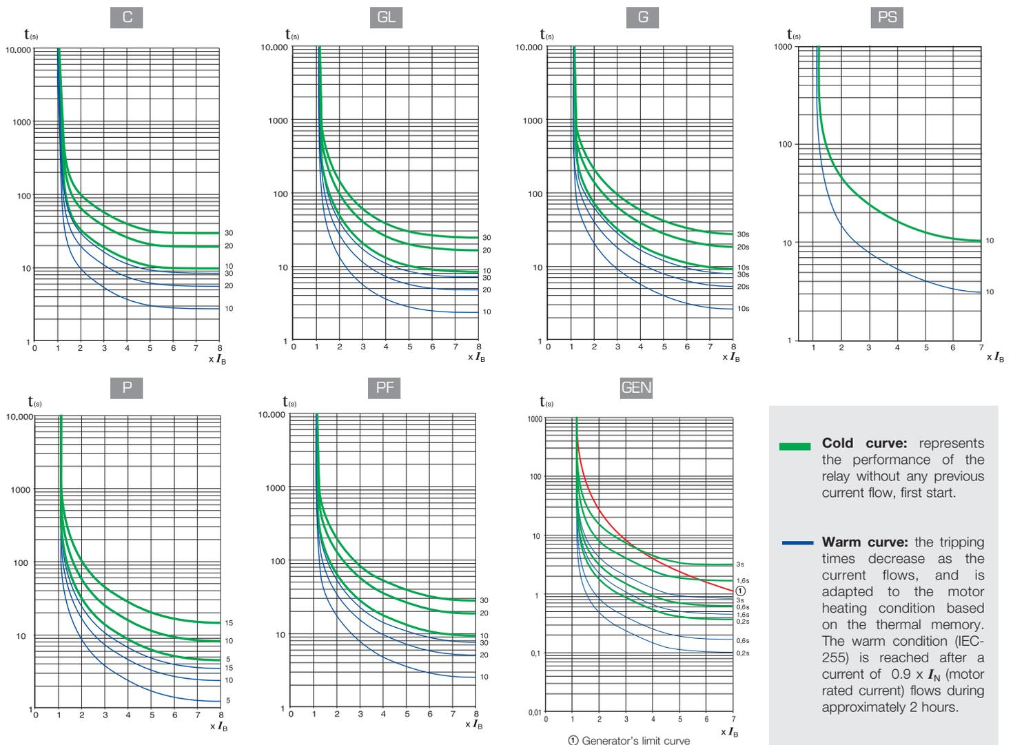
**Cold curve:** represents the performance of the relay without any previous current flow, first start.
