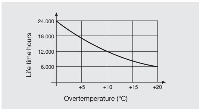
As one can see, a 10°C increase in temperature reduces the useful life of the motor by half.
